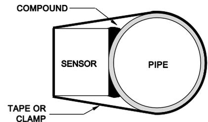
Over time temporary coupling compounds (e.g. Petroleum Gel) may gradually sag away from the sensor resulting in reduced signal strength and finally complete loss of signal. Warm temperatures, moisture and vibration will accelerate this process. Super Lube ® as supplied with the UF D5500 (and available from Micronics Limited) is recommended for semi-permanent installations.
