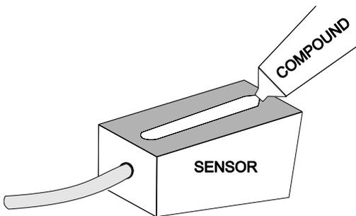
Use the PC4 pipe clamp (supplied) as illustrated on the previous page. Apply Super Lube ® to the coloured face of the sensor. A bead, similar to toothpaste on a toothbrush, is ideal. Do not overtighten (crush the sensor).
