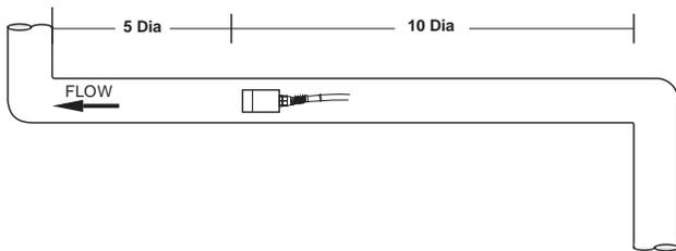
**STRAIGHT RUN REQUIREMENTS** – For best results, the transducers must be installed on a straight run of pipe, free of bends, tees, valves, transitions, insertion probes and obstructions of any kind. **For most installations, ten straight unobstructed pipe diameters upstream and five diameters downstream of the transducers is the minimum recommended distance for proper operation.** Additional considerations are outlined below.
