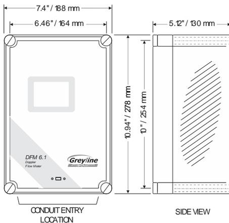
Note: This non-metallic enclosure does not automatically provide grounding between conduit connections. Grounding must be provided as part of the installation. Ground in accordance with the requirements of the National Electrical Code. System grounding is provided by connecting grounding wires from all conduit entries to the steel mounting plate or another point which provides continuity.
